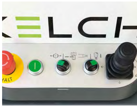
Control panel with joystick to move the CNC axes.
