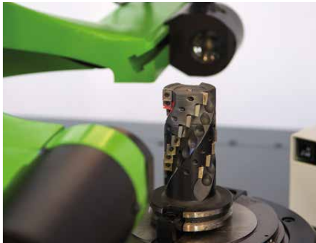
Optics carrier including CCD camera and pneumatic quick adjustment. Optional laser pointer for detection of the cutting edge.
