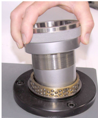
Fig. 3-2: Inserting the receiving sleeve (accessories) into the ball-type nipple (SECA C only)
