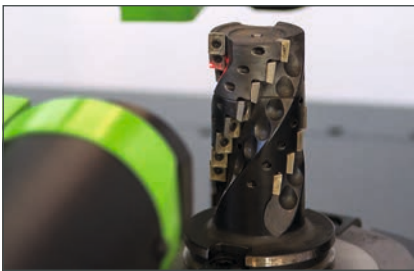
Optics carrier including CCD camera and pneumatic quick adjustment. Optional laser pointer for detection of the cutting edge.
