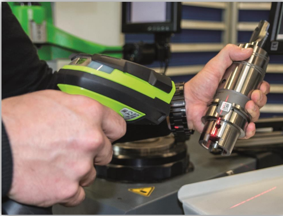
The KELCH QR code is read by a hand-held scanner
