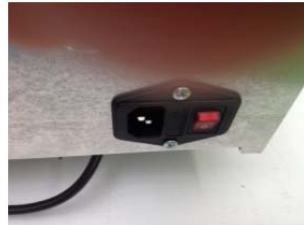
Figure 3: Main switch on the rear side of the presetter
