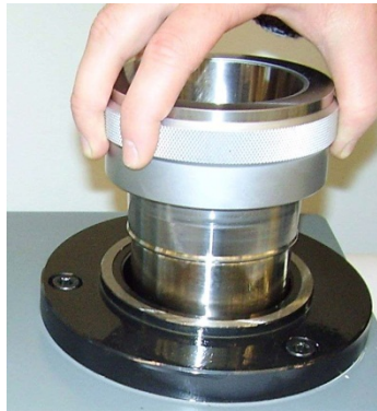
Figure 7: Inserting the tool holder (adapter sleeve) (accessories) into the spindle
