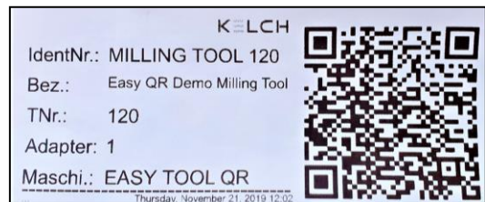
QR label includes tool length & radius along with machine-specific data such as tool life
