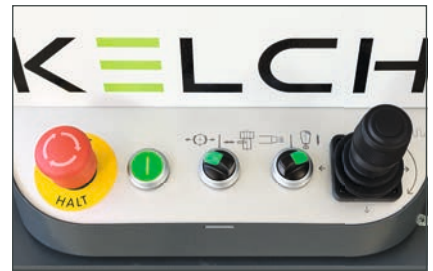
Control panel with joystick for moving the CNC axes
