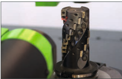
Optics carrier including CCD camera and pneumatic quick adjustment. Optional laser pointer for detection of the cutting edge.
